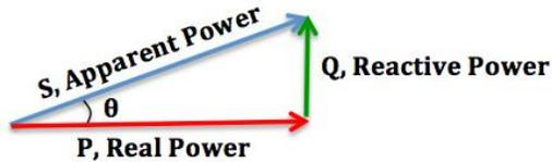
If you know the phase angle between the current and voltage you can calculate the power factor. Power factor is the cosine of the angle between the phase between the current and voltage.
