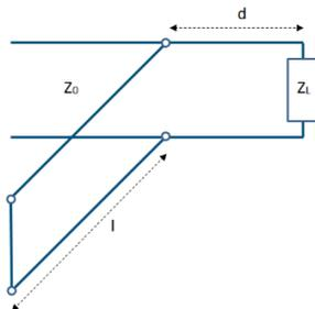
**Stub matches are widely used to match any complex load to a transmission line. They consist of shorted or opened segments of the line, connected in parallel to a line at appropriate distances from the load. The single stub match is a widely used matching circuit.**
