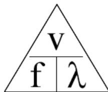
We frequently refer to the frequency bands in amateur radio by their wavelength in meters. For instance, 146 Megahertz (MHz) would be the 2 meter band. Wavelength is easily calculated as using the triangle. Cover the  $\lambda$  in the triangle and you will see it is equal to  $(300) \div (\text{frequency in MHz})$ . To find the wavelength for 146 MHz we would proceed as follows:
