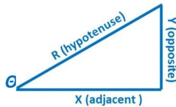
The sides of the triangle are given names from the rectangular coordinate system with the horizontal side called X (also called the Adjacent side) and the vertical side is called Y (also called the opposite side) and the side connecting the X and Y sides is called the Hypotenuse called R in this example. If two of the three sides are known then the third side can be found using the following equation:
