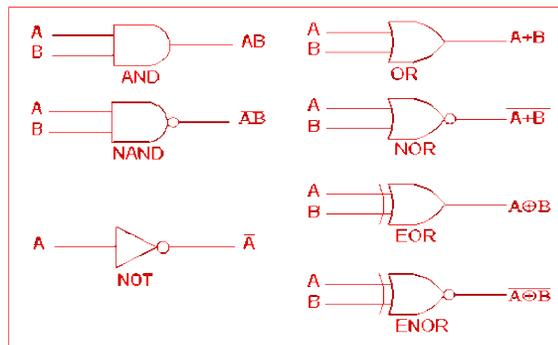
Digital logic devices are used to generate a specific output based one or more input(s). For example:
