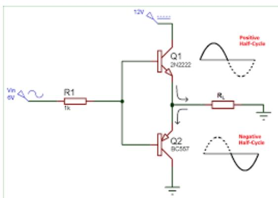
This is a class B push pull amplifier output stage. Each transistor only conducts on one half of the cycle, but they are summed to produce a full cycle. The advantage over a class A amplifier is that there is little or no current flowing when there is no input signal. There will be some loss of signal at the crossover point which will show up as distortion.
