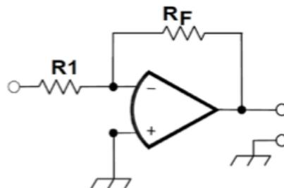
*Gain = feedback resistor ÷ input resistor or Gain = 470 ÷ 10 or 47*
