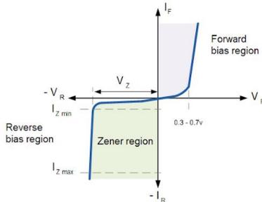
A Zener diode is a diode that when reverse biased will have a constant breakdown voltage vs current flow over a wide range of current. The current must be limited in the Zener region to prevent too much current from flowing which would result in failure of the diode.
