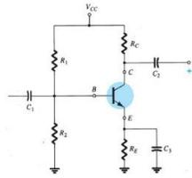
*The series emitter resistor will limit the current flowing when the transistor is biased full on.*
