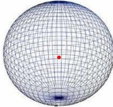
*An isotropic source can be thought of a theoretical single point source with equal power being radiated in all directions. A dipole has + 2.15 dB gain over a theoretical isotropic source.*
